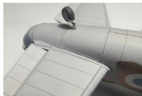
Noter le raccord karman aile/fuselage
